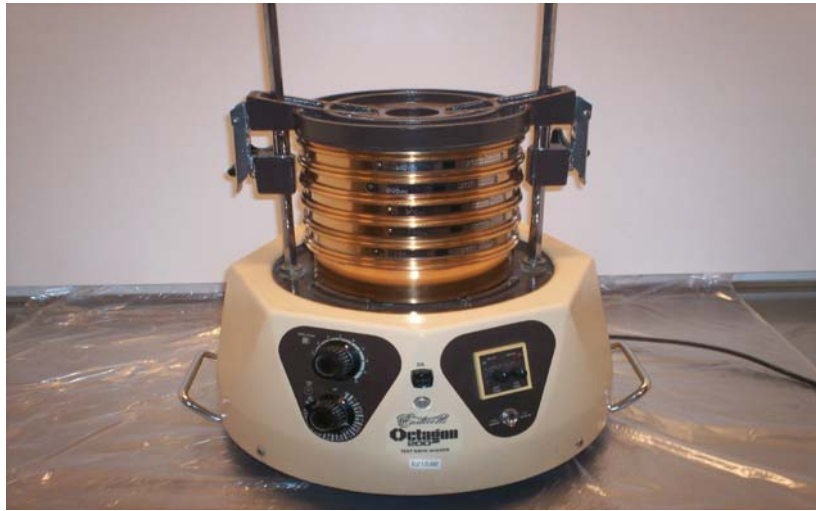
Figure A1: Mechanical Shaker for granulate separation into fractions
