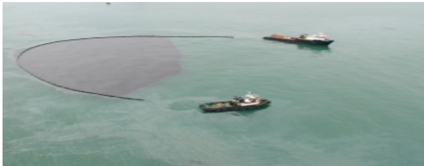
Figure 2.4: Towing Booms at Sea in U Configuration. Source: ITOPF, 2007.
