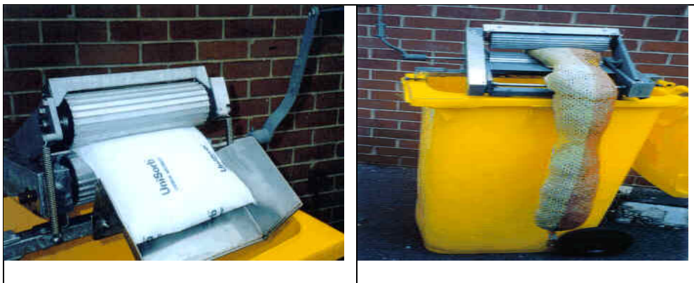
Figure 2.14: Absorbent Hand Wringer for Extracting Oil for Sorbent Re-Use Source: Global Spill Control, Australia.
